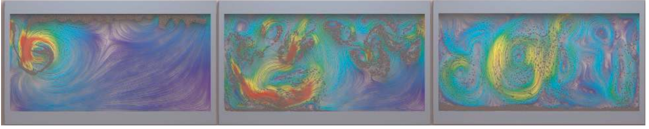
Figure 4.10: Sedimentation 2D : A box of dirt is dropped into a water container, creating interesting vortices before settling down.
