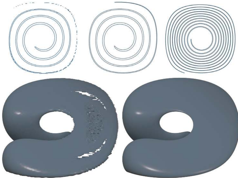
Figure 2.6: (Top) A comparison of (left) particle level set on a 128^2 grid, and (middle) our interface tracking scheme on a 2048^2 grid for a deforming sphere at t = 5 seconds; (right) our scheme at t = 15 seconds. (Bottom) A comparison of (left) particle level set on a 128^3 grid and (right) our method on a 2048^3 grid. For particle level set, near-interface cells use 256 particles. The narrow band level set conserves volume well, over long time periods.
