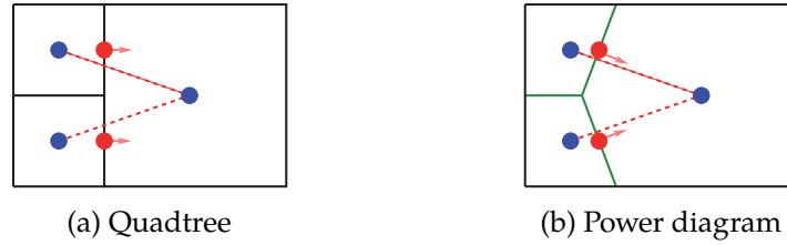
Figure 1.4: Adaptive orthogonality. Left: In quadtree (octrees in 3D), orthogonality cannot be retained; Right: Our power-diagram based discretization restores orthogonality.
