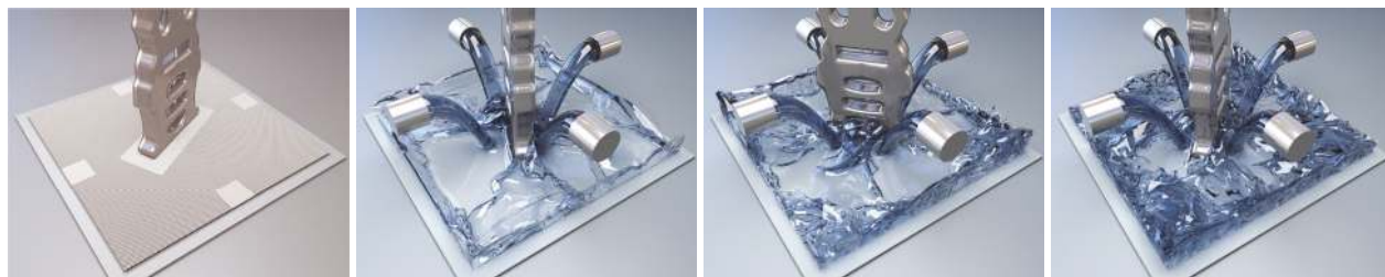
Figure 2.2: Four sources pour water that collides with a kinematic rotating object in a container, with effective resolution 512^3 . The adaptivity pattern, illustrated on the left, continuously rotates with the central spinning object. A narrow band level set with 2048^3 resolution is used to track the free surface.
